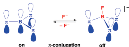
Figure 1. Schematic representation of the switching of \pi -conjugation in the LUMO of boron-based \pi -electron systems: \pi stands for \pi -conjugated moieties.
